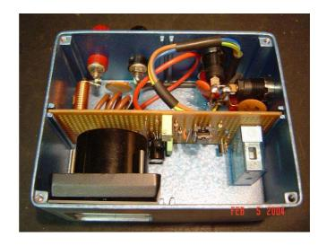
**Meter:** Was a Minipa 5mA ex-fleamarket with deformed spring that needed considerable TLC. A hole was carefully made into the side of the meter window for the BATTERY FULL LED to be pushed in horizontally. Being inside the box and inside the meter, the LED will be quite visible in daylight. The shunt should be of thick wire to carry 5A and prevent it warming up and so altering the reading. It can be seen coiled behind the meter.
